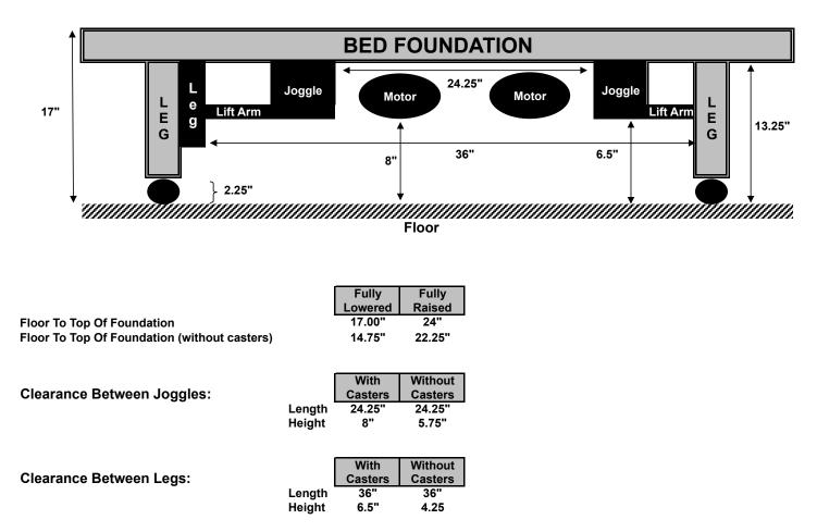
**NOTE>** The hi-lo motor is mounted on the right side of the bed (if you are lying down in the bed). That means that there is more clearance on the left side of the bed (if you are lying down in the bed).
